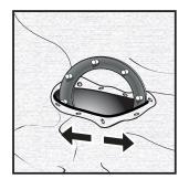
STRETCH WITH CARE without tools, in order to pass inside the flange with its seal
