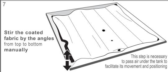
Shake and spread correctly the tank to remove all the folds
